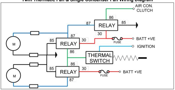
Twin Condenser Fan Wiring Diagram
