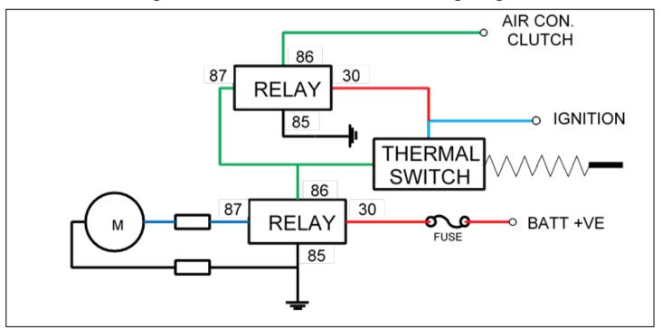
Single Condenser Fan Wiring Diagram
